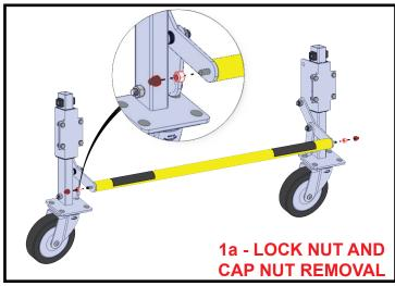
1a. Identify the Wheel Lift bar that needs to be replaced. Remove and discard the cap nuts and lock nuts from both ends using a 7/16" wrench and locking pliers. Then, remove and discard the old yellow bar assembly.
