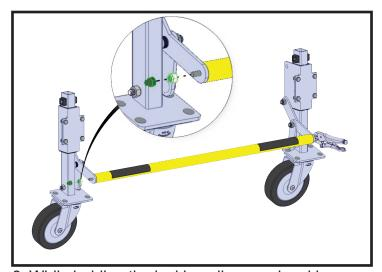
6. While holding the locking pliers, and making sure the labels are facing upward, install a new lock nut, using a 7/16" wrench, then install a new cap nut onto the exposed end of the threaded rod.
