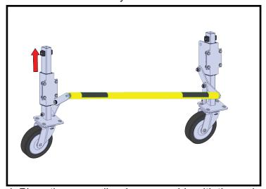
4. Place the new yellow bar assembly with the ends of the threaded rod through the holes in the arms of each wheel assembly. This is easiest when you retract one wheel assembly.
