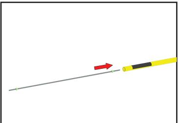
2. Insert the new threaded rod with the two lock nuts on it into the new yellow Wheel Lift bar.
