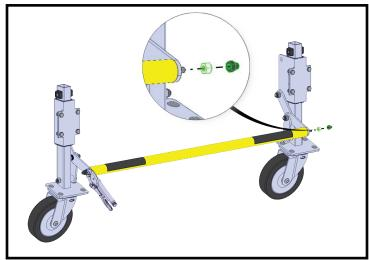
7. Move the locking pliers to the other side, and install the remaining lock nut and cap nut using a 7/16" wrench. Make sure the bar is completely tight and secure before returning the Wheel Lift to service.
