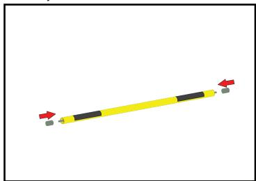
3. Insert the new spacers into each end of the yellow bar and onto the threaded rod.
