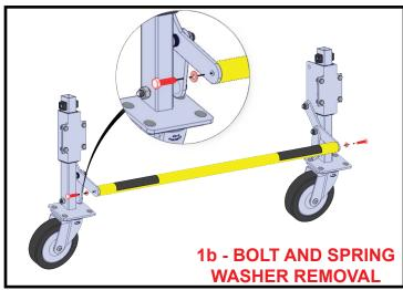
1b. Identify the Wheel Lift bar that needs to be replaced. Remove and discard the bolts and spring washers from both ends using a 7/16" wrench. Then, remove and discard the old yellow bar assembly.
