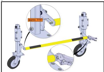
5. Center the threaded rod, where approximately 7/16" sticks out each side, then hold one end of the threaded rod in place with a pair of locking pliers.
